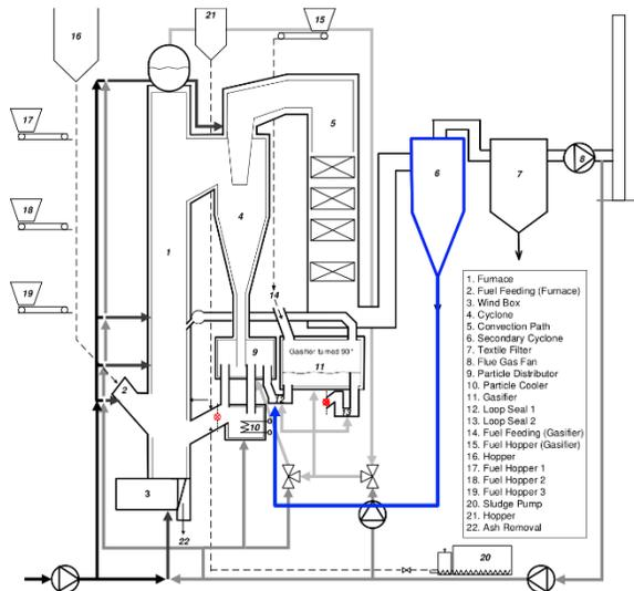
**Figure 1:** Layout of the Chalmers gasifier.
