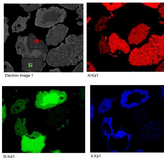
**Figure 3.** SEM/EDX image of the bauxite - quartz sand mixture
