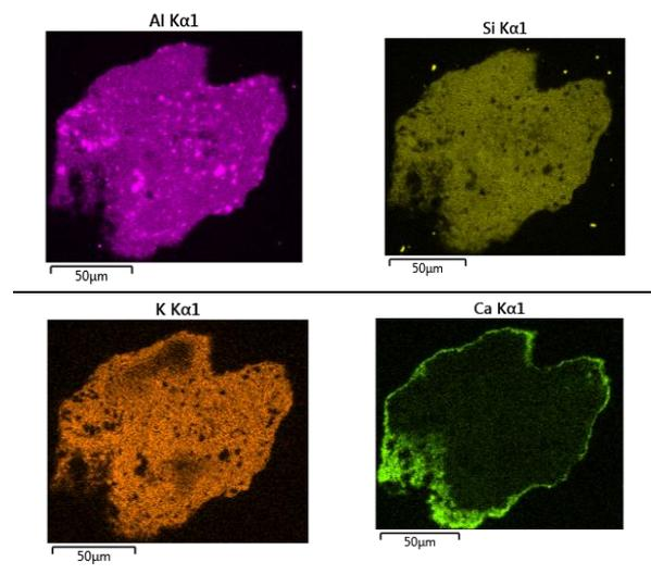
**Figure 2.** SEM/EDX image of bauxite particle enriched by ash elements
