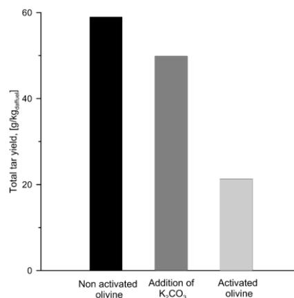
**Figure 4.** Total tar yield including Benzene and one 1-ring in g/kg<sub>fuel</sub> before, after K<sub>2</sub>CO<sub>3</sub> addition, and after K<sub>2</sub>CO<sub>3</sub>+S addition
