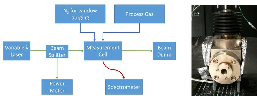
Fig. 3: Left: Scheme of the lab setup for the fundamental research on PAH compounds. Right: Measurement Cell. View from the laser, gas flowing from left to right, spectrometer out on top.
