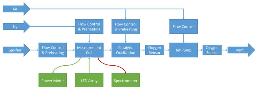
Fig. 5: Scheme of the work-in-progress on-line analysis tool that will be placed into operation in early 2016.
