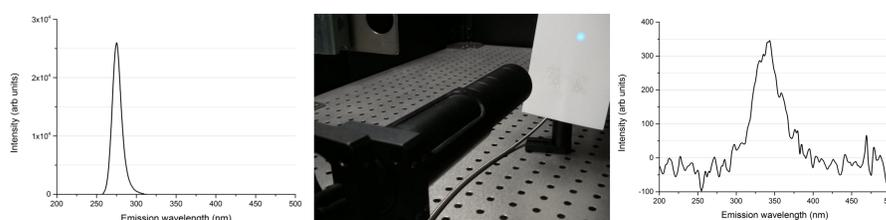
Fig. 6: Left: emission spectra of a 275 nm 1 mW UV-LED. Middle: focused UV-LED (dot diameter approx. 10 mm). Right: Corresponding emission spectrum of naphthalene in N<sub>2</sub> carrier gas at 300°C.
