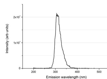
Fig 2: Emission spectrum of fluorene excited with 240 nm laser light.
