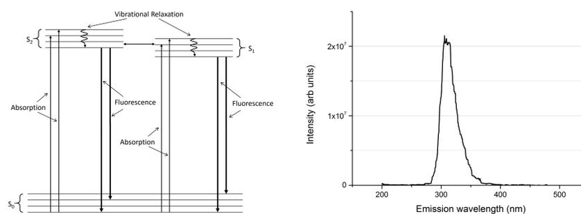
Fig 1: Scheme of the Jablonski-diagram showing the principle of absorption and emission of photons leading to fluorescence [2].
