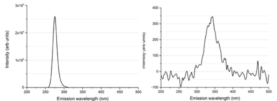
Figure 1: Emission spectrum of a 275 nm 1 mW UV-LED (left) and the corresponding emission spectrum of naphthalene excited by this wavelength
