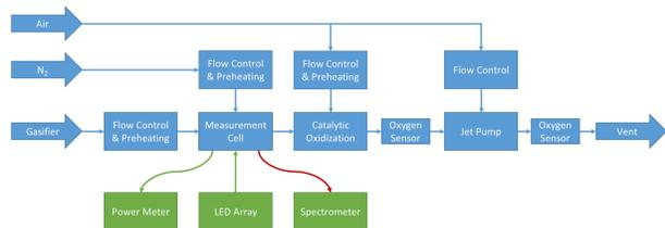
Figure 2: Setup of the measuring device
