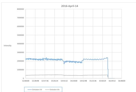
Figure 3: Course of the emission with <300 nm excitation wavelength; the change in gasification conditions at 13:55 and 14:52 have a significant effect on the detected signal.
