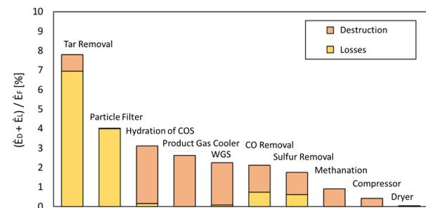
Figure 4: Exergy losses and destruction in the unit operations downstream of the gasifier in a biomass to SNG plant.
